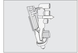
Hold the magnets at the side and pull forwards to release the unit.
